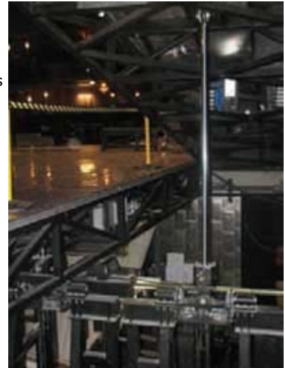
One of two cylinders pivots a stage platform upward. The cylinder's long stroke required careful evaluation of its rod's buckling strength. Integral linear displacement transducers on cylinders provide continuous feedback of position for synchronized control of multiple electrohydraulic axes.
